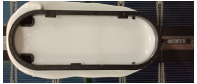
Junction Box opened view(BOM 2)
