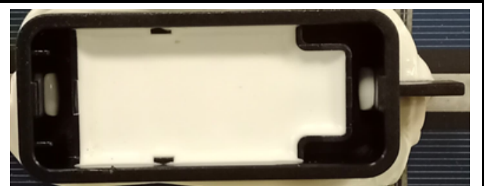
Junction Box opened view(BOM 1)
