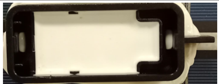
Junction Box opened view(BOM 1)
