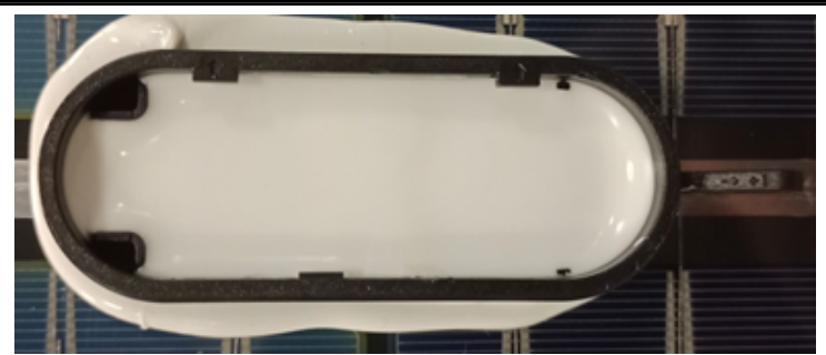
Junction Box opened view(BOM 2)
